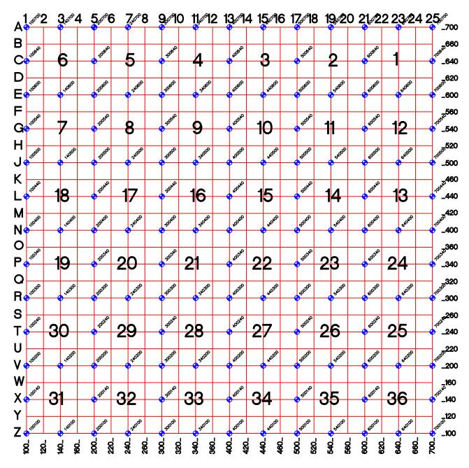
The historical index methodology for the corner records in Ada County has been where each corner certificate is identified by an alphabetical- numerical coordinate number which is derived from the system shown on the above township diagram.
